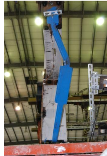
KBRF with out-of-plane buckling
